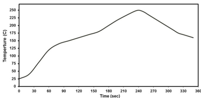
**Typical HiP Reduction Profile for No Clean Flux**
