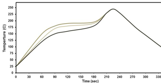
**Typical Void Reduction Profiles For No Clean Flux**
