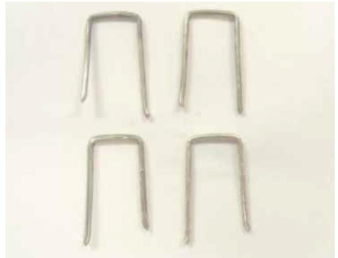
**FIGURE 1.** Hot dipped test specimens after bending.
