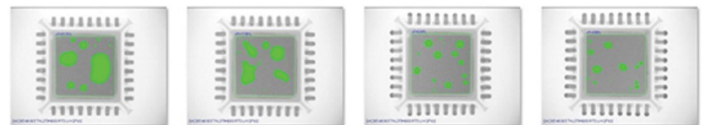
FIGURE 1. Void reduction on BTC ground pads as a result of changing I/O aperture design while maintaining the same ground pad aperture design on the original experiment.
