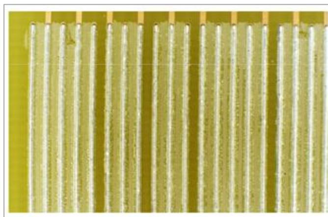
**Figure 5.** Paste 55 post-thermal shock, showing evidence of delamination
