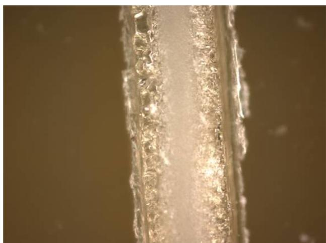
**Figure 12.** Enhanced close-up of flux residue and delaminated coating layers.
