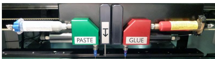
FIGURE 2. Solder paste dispenser mounted inside stencil printer.
