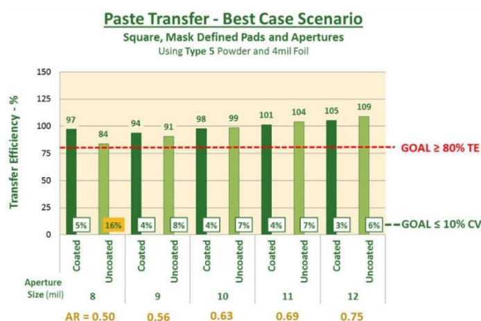
FIGURE 2. Transfer efficiency and CV of type 5 powder at various area ratios (AR)
