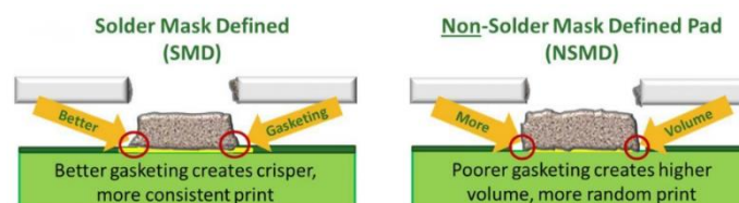
FIGURE 1. Effect of pad definition on solder paste print quality
